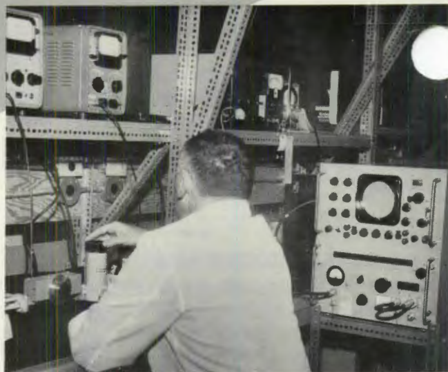
Mr. Joseph Moss checks frequency of a Klystron Oscillator in the Microwave Calibration area.
