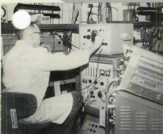
SSgt Riley calibrates a USM-44 in the Electronic Calibration area, using test equipment mounted on roll-away carts.
